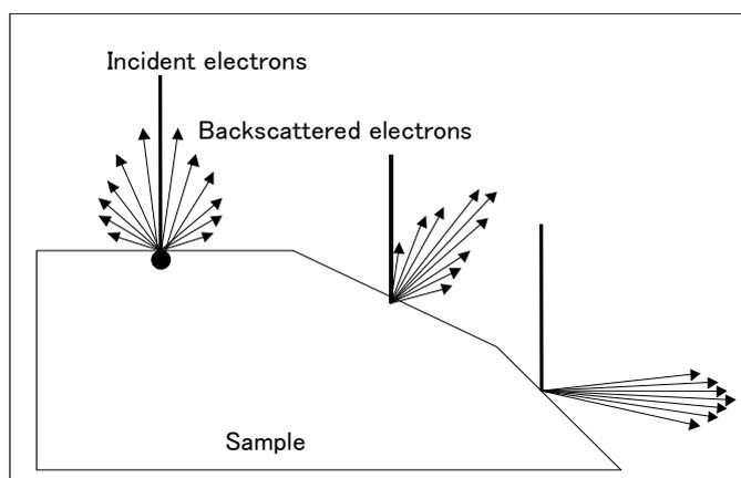
Figure 1. Backscattered electron emission angles
