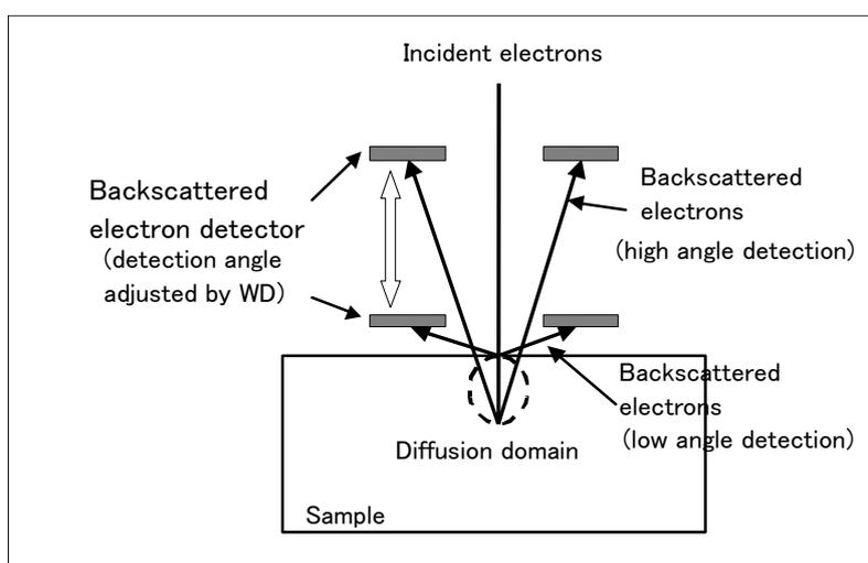
Figure 2. Detector positions and angles
