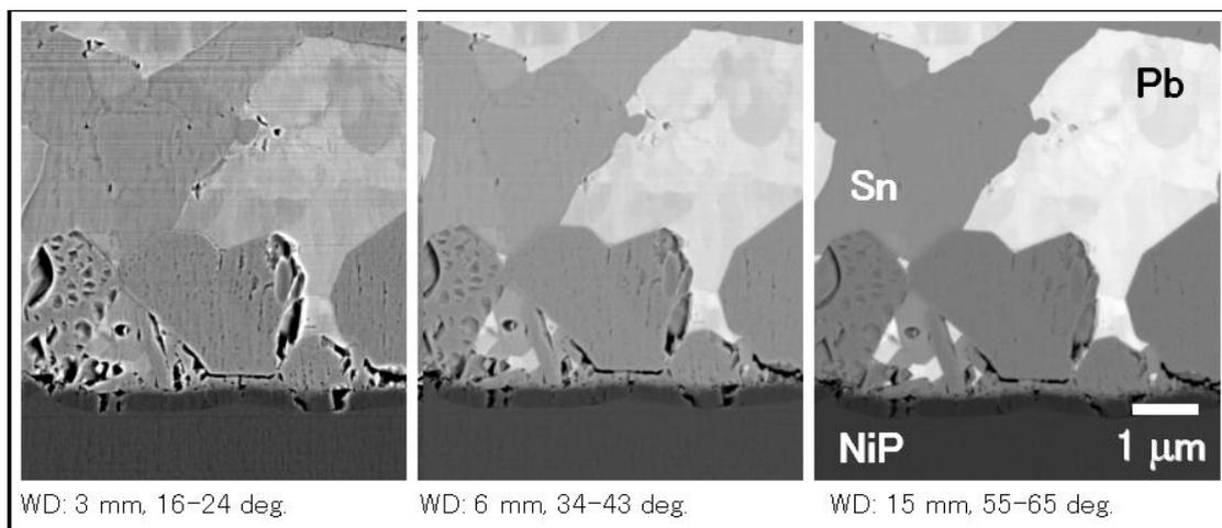
Figure 3. Backscattered electron images acquired at different detection angles
